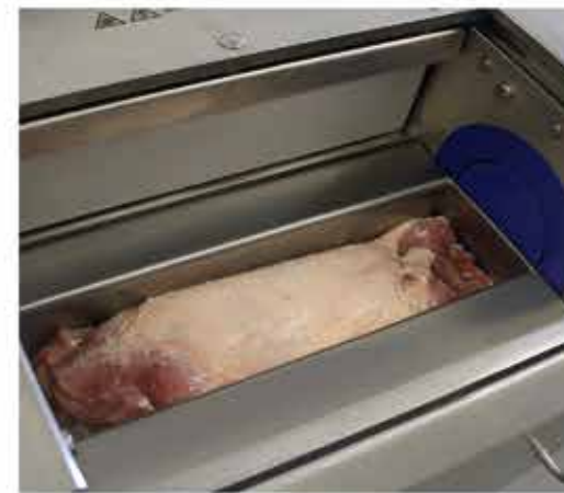
High power press system to shape and form the product for stuffing into netting or casings or both.
