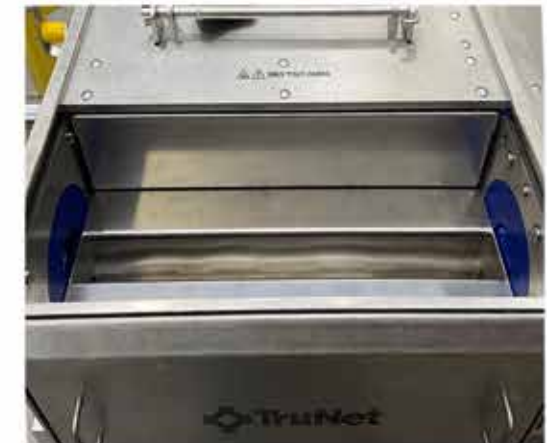
Extended 800mm press chamber designed to press whole loins into slicing logs.
