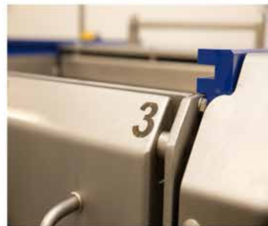
Manufactured fully from Stainless Steel AISI 304 all non Stainless Steel parts are food grade and approved for use in the food industry.
